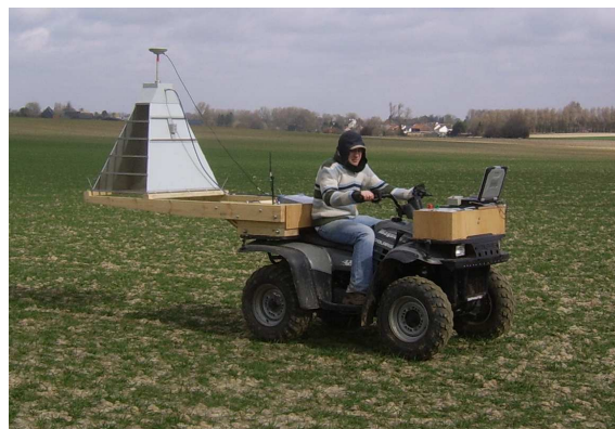
Figure 4: Four-wheel motorcycle holding the GPR system constituted of a horn antenna linked to a vector network analyzer, the DGPS device and the laptop. Picture taken on the 23 th of March 2009 in a barley field near Walhain, Belgium.
